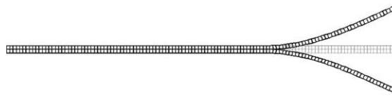
Fig. 14. Original and deformed (5 mm opening) models of the DCB test specimen using a 120 \times 2 mesh.
